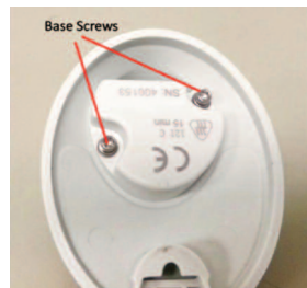
Figure 1: Screws on base connecting to body
