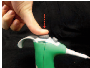
Figure 3: Plunger Button Reattachment
