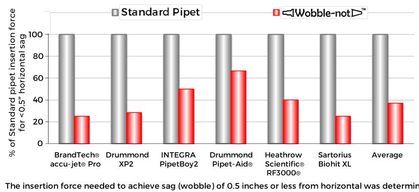
The insertion force needed to achieve sag (wobble) of 0.5 inches or less from horizontal was determined using Standard and Wobble-not serological pipets with a variety of pipet controllers. The force for the Standard Pipet using each controller was set at 100% and relative % force with Wobble-not determined. With every controller tested, Wobble-not pipets required less force for the low level of pipet wobble.
