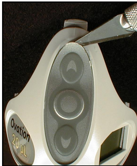
Figure 3 Peeling Keypad assembly from Base
