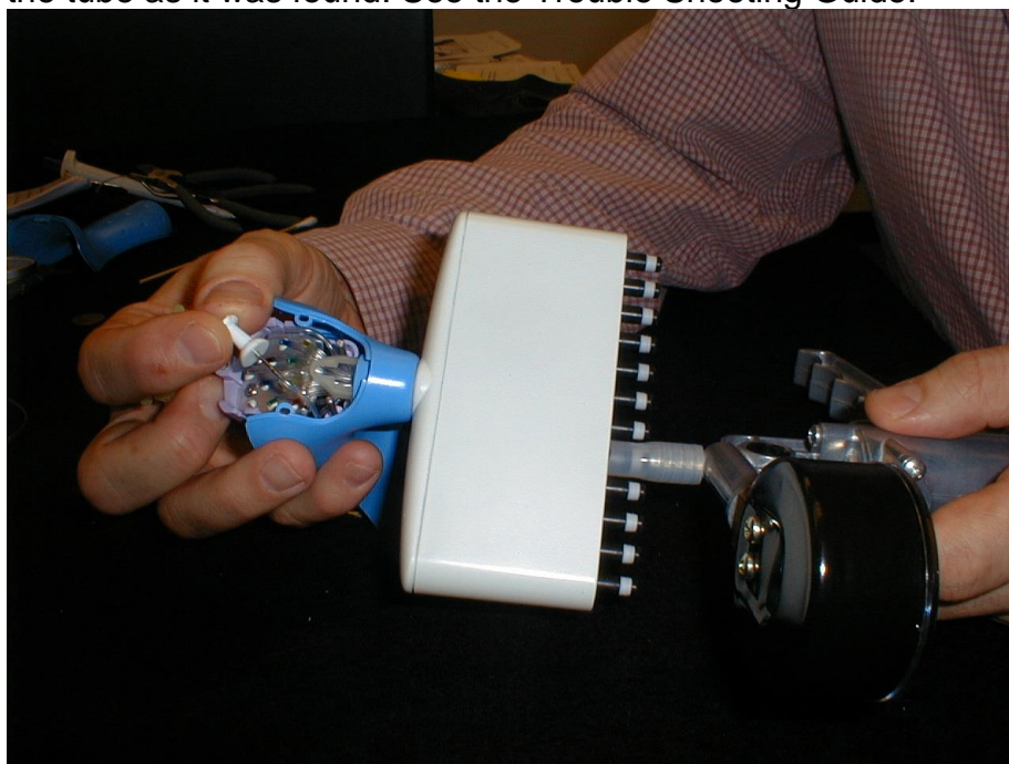
Figure 10 Removing tube from top plate and plugging with push pin
