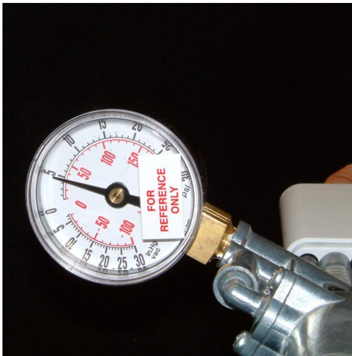
Figure 12 Pressure Pump at 4 psi
