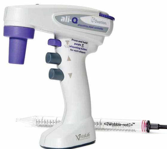
experimental outcomes. A device that automatically accounts for these factors saves valuable time and reduces the risk of error. The innovative ali-Q™ design uses computer-controlled sensors and valves that automatically detect changing environmental conditions and subsequently adjust volume settings to deliver the correct volume with each semi-automatic dispense.
