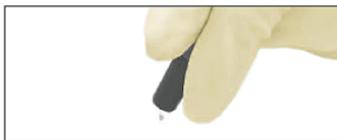
8. Re-insert the rubber nozzle plug into the front end of the nozzle. The end of the plug without side ridges is inserted first. Press in until plug is even with surface edge of the nozzle. If filter is not completely seated, the plug will extend beyond the end of the nozzle. Remove plug and firmly seat filter with insertion tool.
