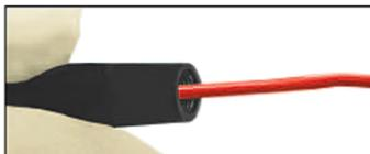
5. Pick up a new nozzle filter with tweezers and place it into the tip end (non-threaded) of the nozzle. The end of the filter with the visible ridge should be inserted first.
