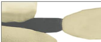
9. Place rubber tubing onto the nozzle, and screw the nozzle onto the pipette in a clockwise direction. Firmly tighten and remove tubing from nozzle. Re-install ejector sleeve.
