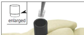
6. Use the filter insertion tool to push the filter into position. Firmly press down until the filter is pushed to the bottom of the nozzle.
