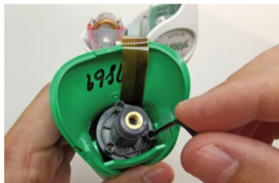
Figure 3: Loosen 3 captive screws
