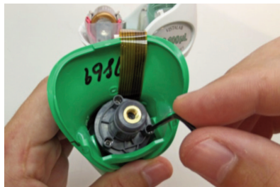
Figure 12: Tighten captive screws
