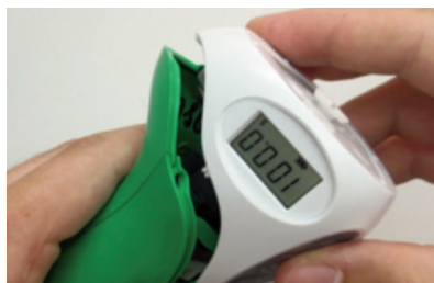
Figure 13: Put the base back onto the pipette
