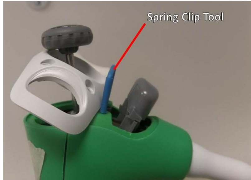
Figure 4: Ejector sleeve pushed inward, ejector spring restrained
